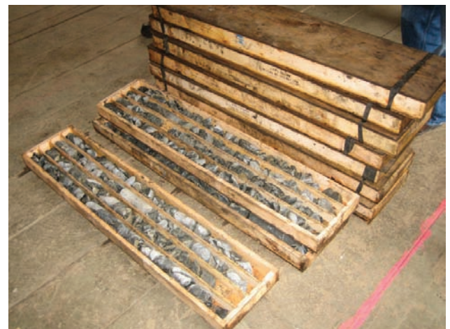
New Drill Core Samples
