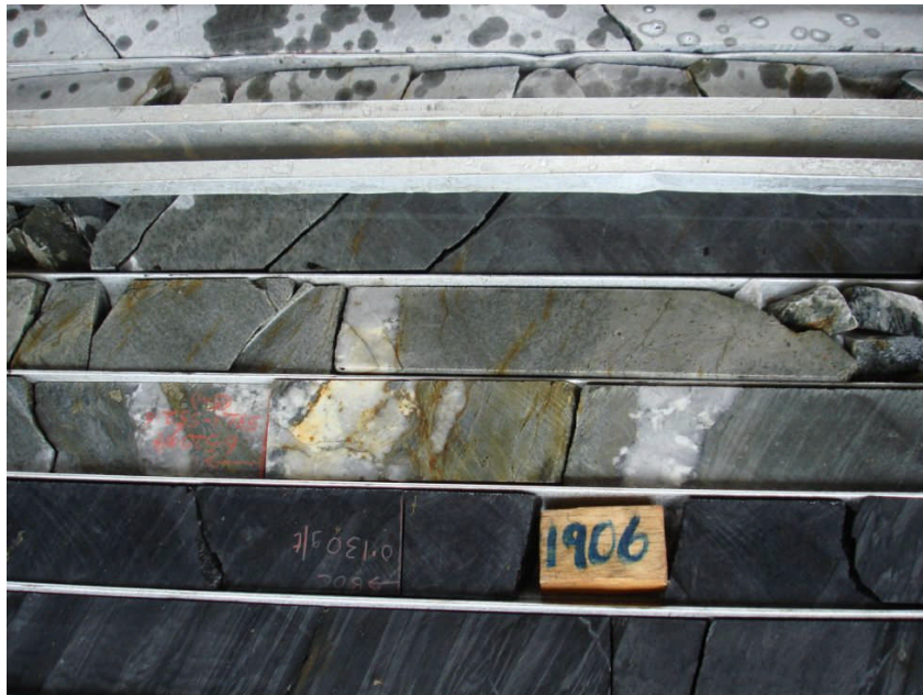
A mineralized section from the Obotan drill core. Source: Fundamental Research Corp.
