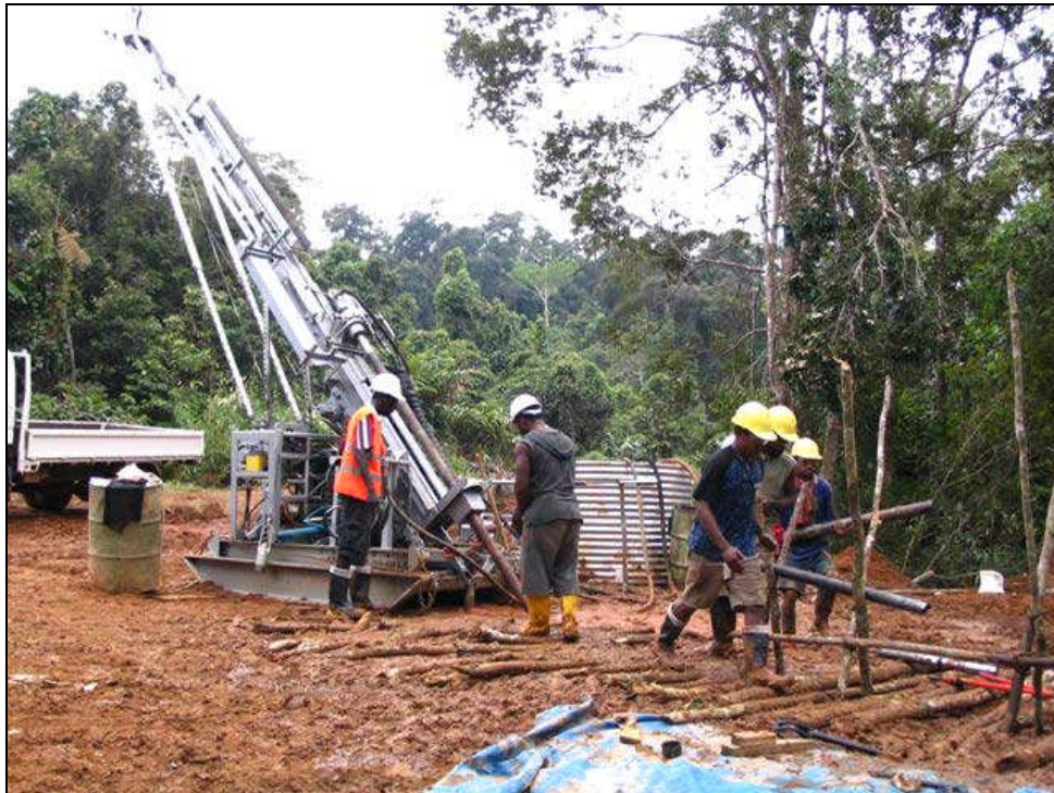
Diamond drilling with a company owned rig on the Sinivit property.
