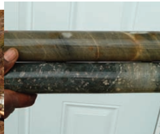
Two types of altered feldspar porphyry (favorable for gold mineralization) encountered at Granada in Phase 2.
